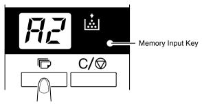
Press the Memory Input key to store the currently selected interval setting of the Cycle Print Mode into the memory.
